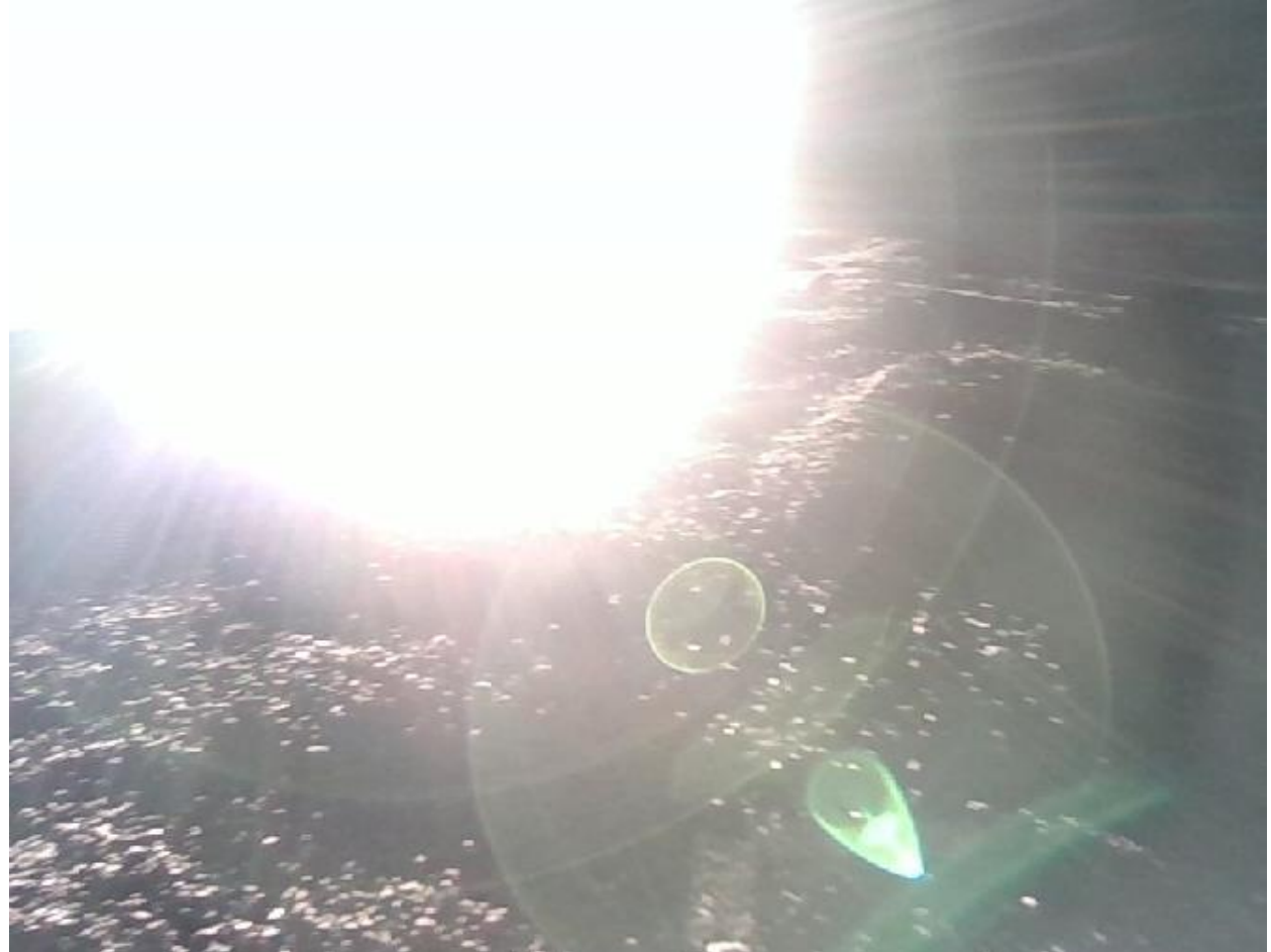
Figure 28 – Lens flares in visual odometry camera
